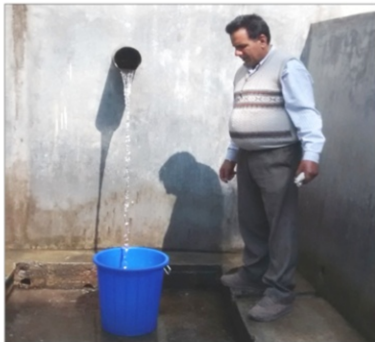
Fig. 4.1 Discharge measurement of a free flow spring
