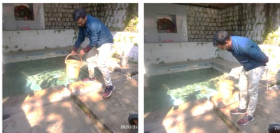
Fig. 4.2 Discharge measurement of a Seep type spring
