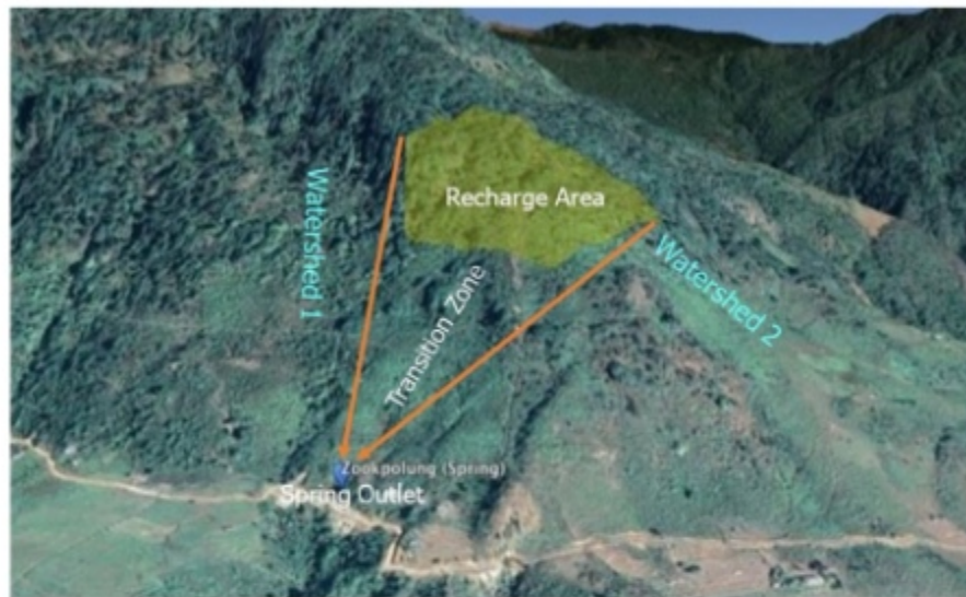
Fig. 2.11 Different components of the spring system
