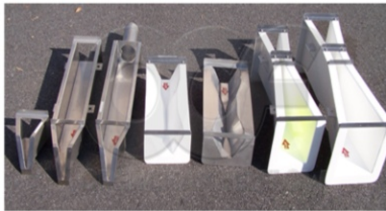
Fig. 4.3 Different shapes flume appropriate to the shape of spring openings
