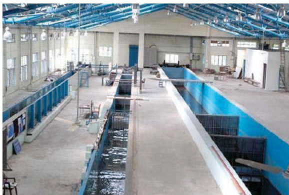
View of Physical Model at CWPRS showing placement of existing weir and proposed barrage
