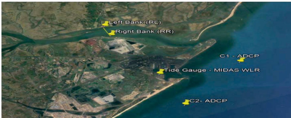
Field data collection for Water Currents (locations C1 and C2) and Water Level was carried out using Acoustic Doppler Current Profiler and Tide Gauge, respectively
