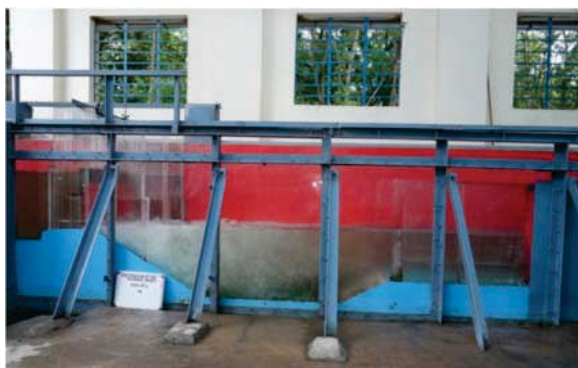
2D Hydraulic model studies for Polavaram Irrigation Project for assessment of discharging capacity at left flank head regulator; views of Stilling Basin and Vortex formation in front of gates
