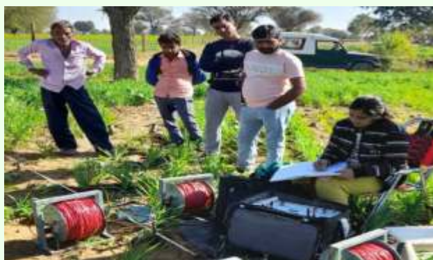
Geophysicist of CGWB, WR, Jaipur, conducted VES at Khatoo village, Danta Ramgarh, Sikar district, Rajasthan.
