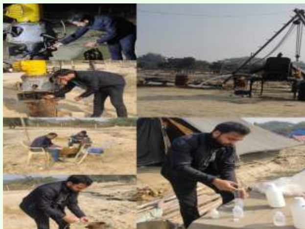
Scientists of CGWB, NR conducted Step Drawdown Test at variable discharge and Aquifer Performance test at 1268 LPM Discharge for determination of Aquifer Parameters and Chemical Quality of Aquifer Group II at Thanagaon, Kothawan Block, Hardoi District under NAQUIM.
