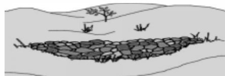
Construction of Gully Plugs Units: 2 No. of Beneficiaries: 85 Water conserved (in Million litres): 0.25
